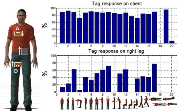
Figure 46: Channel reliability  $\alpha$  for several postures, expressed in term of percentage of answer with the antennas in vertical polarization.
