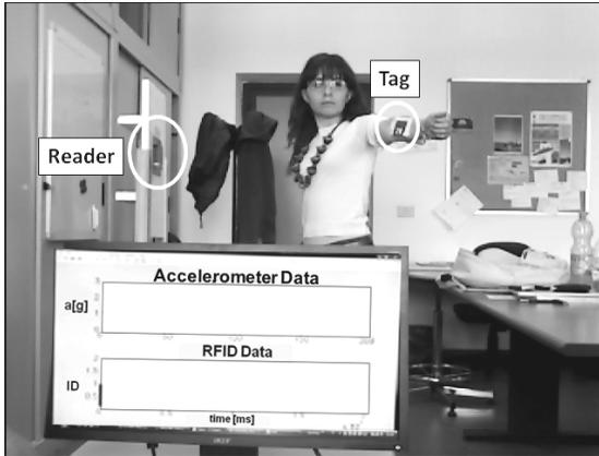
Figure 53: Measurement setup comprising the short-range reader, the RFID tag and the LIS302DL accelerometer placed beside the tag. Both the RFID motion sensor and the accelerometer are placed on the arm. The MEMS accelerometer data is transmitted via a WIFI module.
