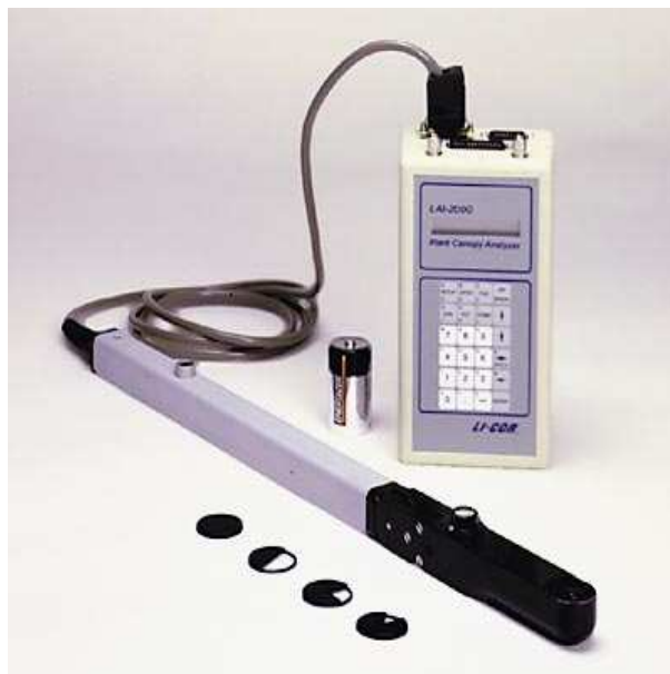
Figure 3.4: LI-COR LAI-2000 instrument with the sensor used in LAI measurements.
