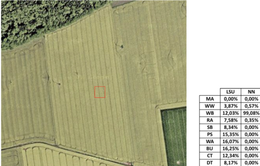
Figure 4.15: High resolution image and abundances matrix of a pixel covering entirely a winter barley area (MA: Maize; WW: winter wheath; WB: winter barley; RA: rape; SB: sugar beet; PS: pasture; WA: water; BU: built-up area; CT: coniferous trees; DT: deciduous trees)
