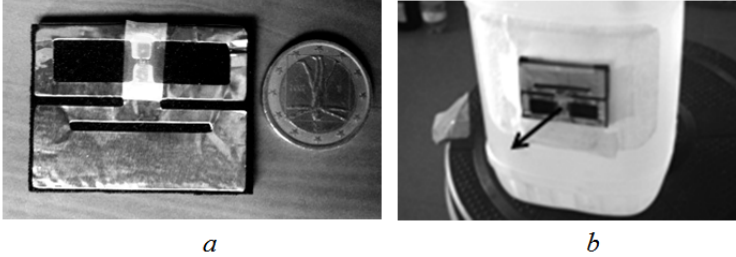
Figure 4.12.: RFID miniaturized wearable aluminum prototype, over a 3mm EPDM black foam having dimensions as reported in Fig. 4.11 and mouth and whisker parameters c=29\text{mm} , n=18\text{mm} . a) Top view of the prototype; b) prototype placed on high lossy laboratory phantom. The arrow indicates the direction of realized gain measurements.
