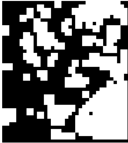
Figure 13.9. Correlation mask achieved by setting the threshold value of the G function correlation to 0.75.
