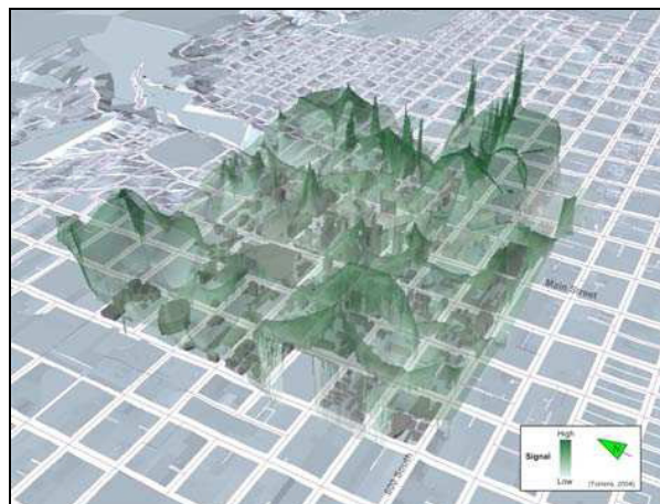
Fig. 2.15; Spatial indicators: intensity of the WI-FI signal of Internet – continuous indicator in three dimensions [Nadia Amoroso, 2010].
