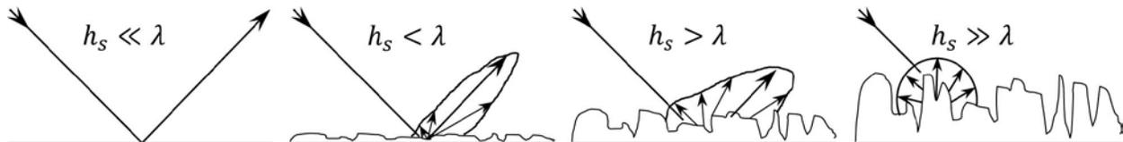
Figure 2.12. Backscatter behaviour over surfaces of varying roughness relative to the incident wavelength.
