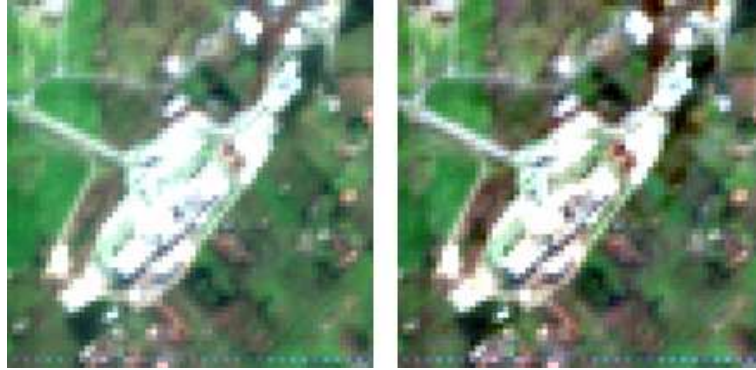
Figure 3.7: Effects of adjacency correction. Particular before the correction (on the left) and after the correction (on the right)
