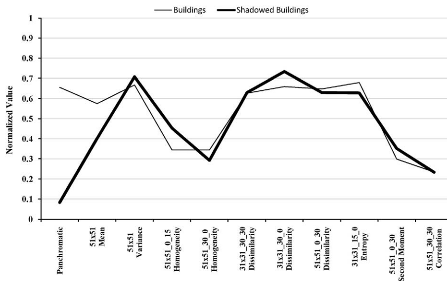
Fig. 11. Normalized textural values of the most contributing features and panchromatic band of the Rome case for shadowed and non-shadowed pixels of buildings (including also apartment blocks and towers). The variance of shadowed buildings is slightly higher than non-shadowed buildings, while homogeneity shows an inversion of the trend between shadowed and non-shadowed buildings using a larger step size.
