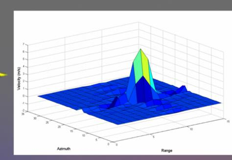
3) Azimuth velocity estimated with a bank of velocity azimuth filter, analyzing the IRF of the moving scatterer.
