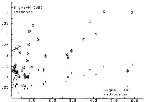
Fig. 5. High frequency rms field amplitude fluctuations  $\sigma_H$  versus low frequency rms fluctuations of atmospheric brightness temperature  $\sigma_{LR}$  for the same segments of the eight events as in Fig. 4.
