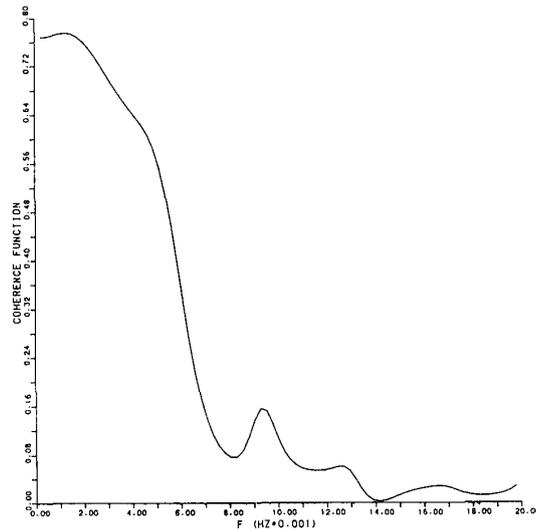
Fig. 3. Coherence function between field amplitude fluctuations received by the 3-m antenna and the atmospheric brightness temperature fluctuations for event on August 8, 1979, 12:00-14:00 GMT.
