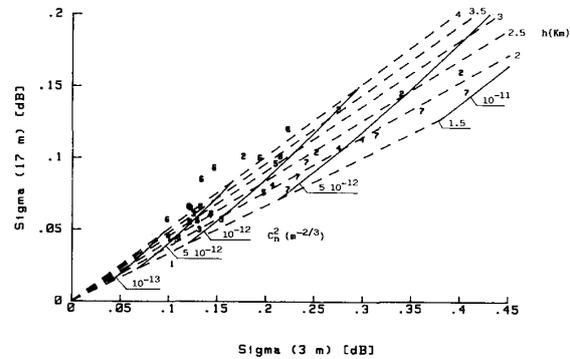
Fig. 6. High frequency rms field amplitude fluctuations received by the 17-m antenna versus the 3-m antenna ones for the same segments of the eight events as in Fig. 4. Theoretical curves for constant turbulent slab thickness  $h$  (broken lines) and for constant  $C_n^2$  (continuous lines) are also shown.
