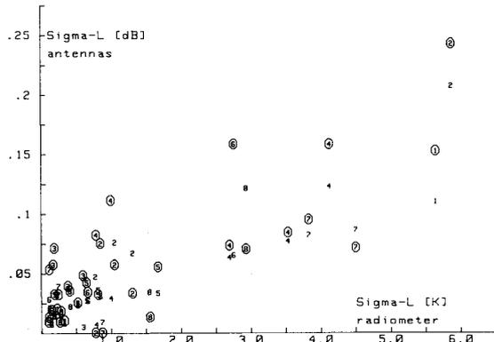
Fig. 4. Low frequency rms field amplitude fluctuations  $\sigma_L$  versus low frequency rms fluctuations of atmospheric brightness temperature  $\sigma_{LR}$  for individual 24 min segments of eight long duration events, numbered 1 to 8. Circled numbers refer to 3-m antenna data, others to 17-m antenna data.
