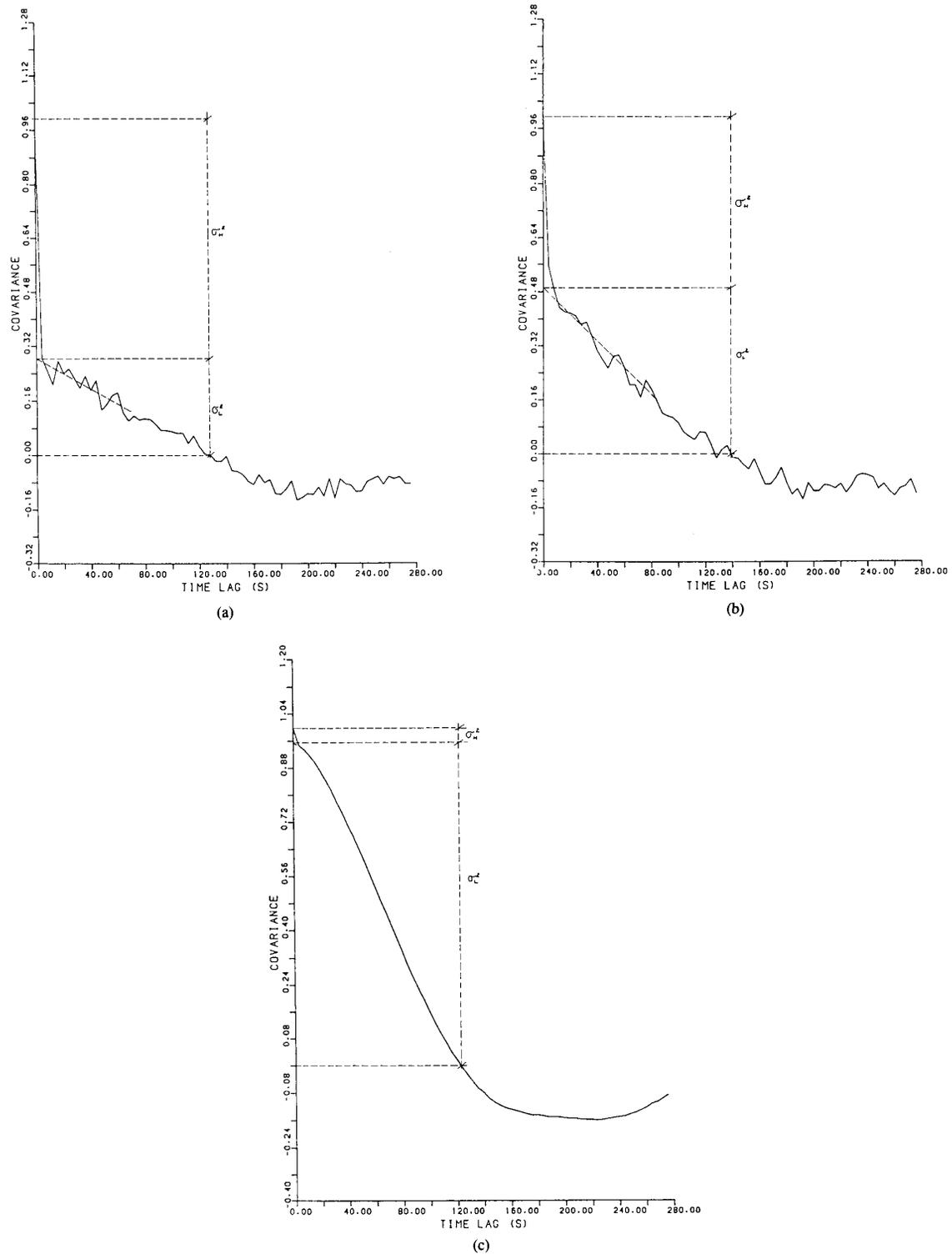
Fig. 2. Autocovariance functions of fluctuations for event on August 8, 1979, 12:00–14:00 GMT. (a) Field amplitude received by 3-m antenna. (b) 17-m antenna. (c) Atmospheric brightness temperature.
