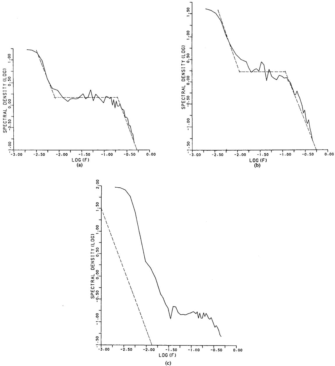
Fig. 7. Spectra of fluctuations for event on August 8, 1979, 12:00–14:00 GMT. (a) Field amplitude received by 3-m antenna. (b) Field amplitude received by 17-m antenna. (c) Atmospheric brightness temperature. Lines with  $-8/3$  slopes are also shown.
