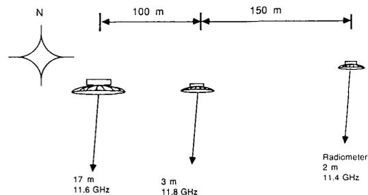
Fig. 1. Schematic representation of OTS beacon and radiometer antennas at the Fucino ground station.
