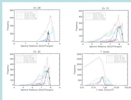
Statistical distribution computed for the three considered channels (CH 28, CH 31, CH 32) and for the Ash total mass BTD results.
