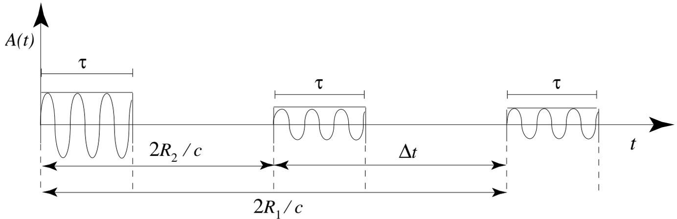
$$\Delta t = \frac{2R_1}{c} - \frac{2R_2}{c} = \frac{2(R_1 - R_2)}{c} > \tau$$
